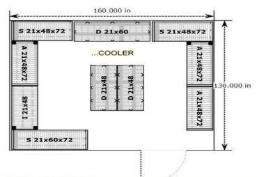
...Elements 4-Shelf units 21"D x 72"H using Starter Kits w/Add-On units. 60" unit has dunnage stand for extra support. 3 each Dunnage Racks
