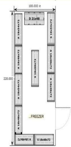
... Elements 4-Shelf units using Starter Units & Add-On units. 18"D x 72"H. All 54" units have a dunnage stand under bottom shelf for extra support
